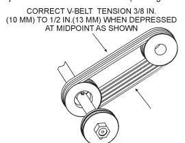
Figure 47. V-Belt Adjustment/Tension
